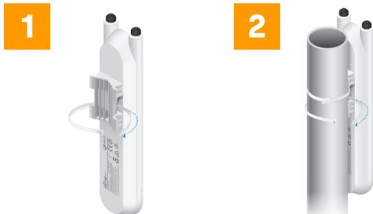
1. Insert a Zip Tie through the slot of the mount bracket on the back of the UniFi AP.
